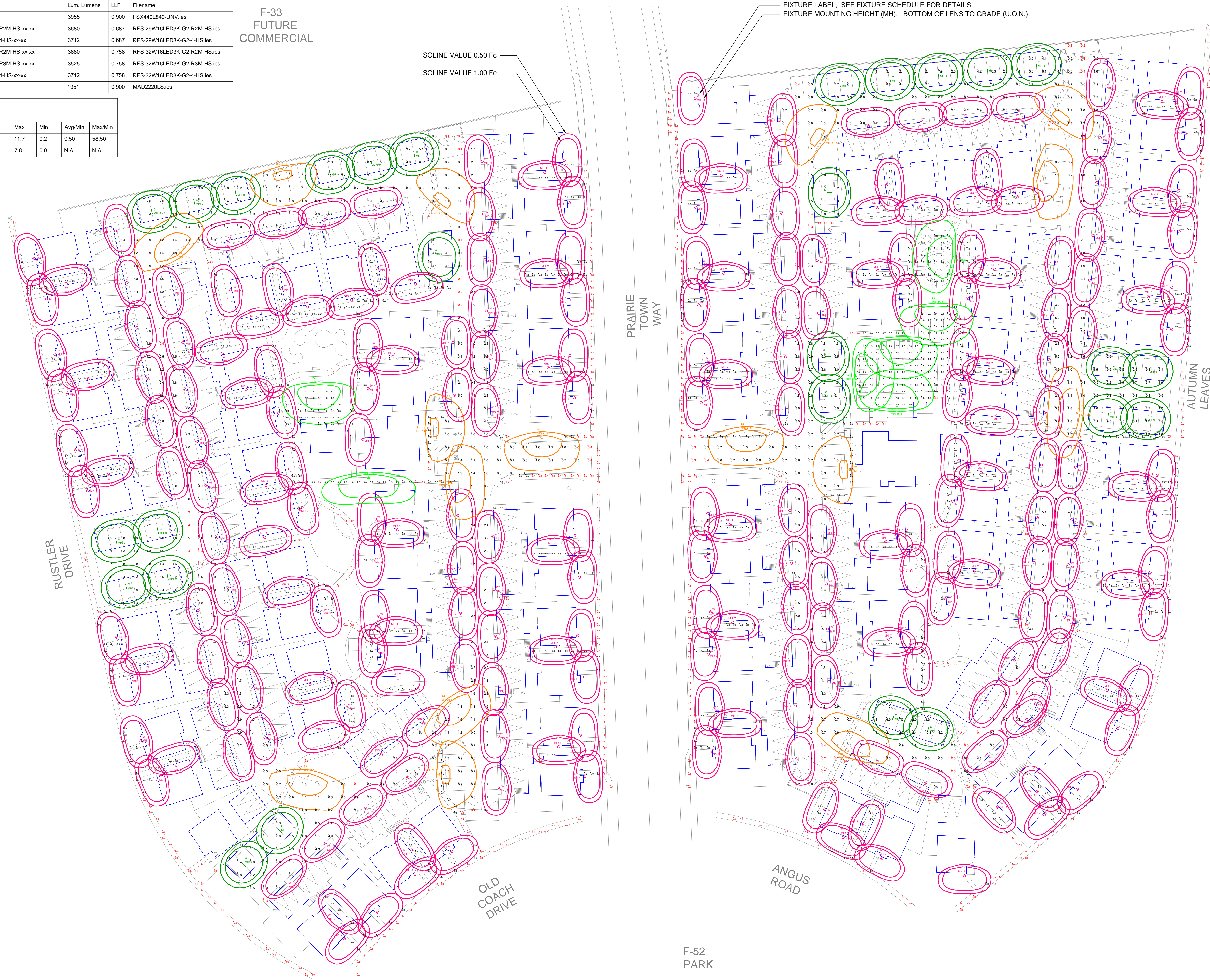
LIGHTING PLAN - PHOTOMETRIC ANALYSIS - LAYOUT VERIFICATION SCALE: 1" = 30'-0" (ALL VALUES SHOWN ARE MAINTAINED HORIZONTAL FOOTCANDLES AT FINISHED GRADE, U.O.N.)
